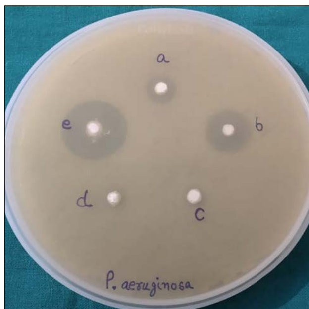
Figure 2. Zones of inhibition representing antibacterial activity of test materials; a, b, c, d, e, against p. aeruginosa
