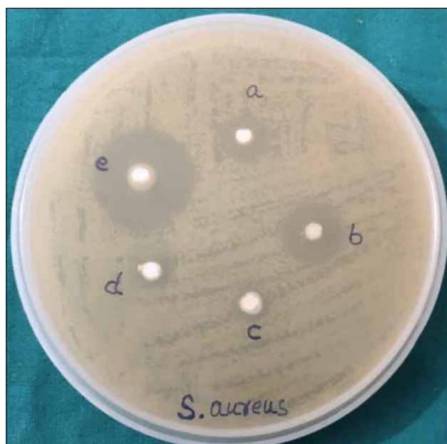
Figure 3. Zones of inhibition representing antibacterial activity of test materials; a, b, c, d, e, against S. aureus
