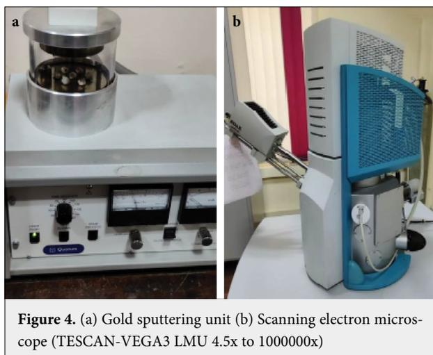
**Figure 4.** (a) Gold sputtering unit (b) Scanning electron microscope (TESCAN-VEGA3 LMU 4.5x to 1000000x)
